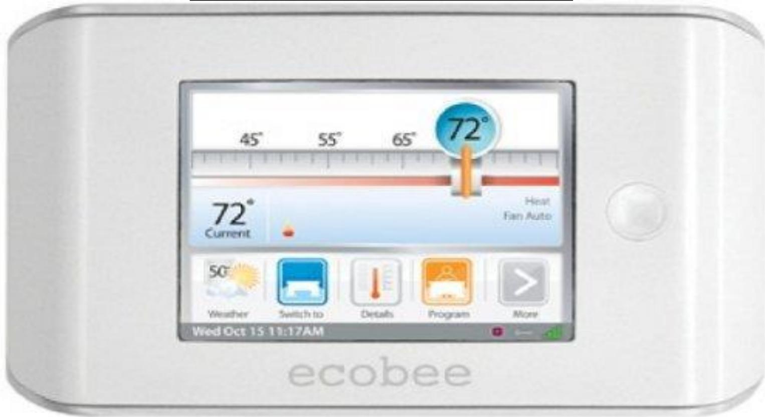
Smart thermostats, such as this Ecobee, do far more than just schedule. They have advanced control algorithms such as optimum start/stop and currently offer free data collection and storage. These can be accessed remotely via smart devices and have customizable reset abilities and access.
