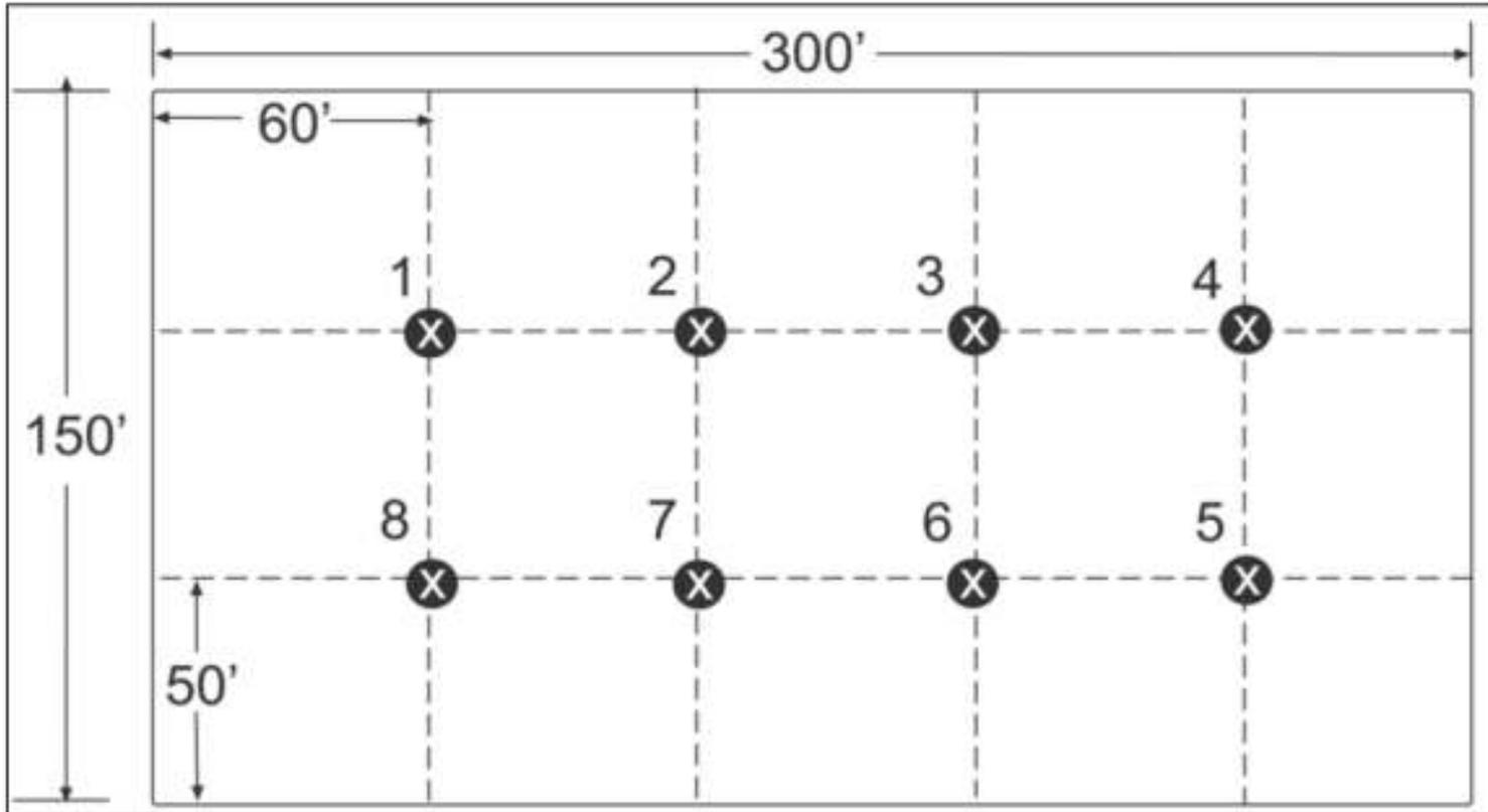
Sample layout grid for a 150 ft x 300 ft lagoon that identifies sample points where sludge depth will be measured.
