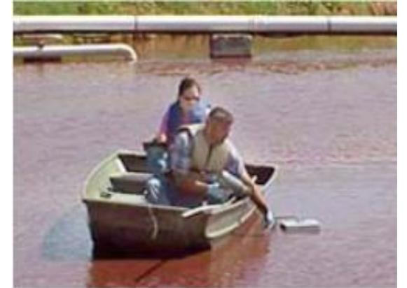
Using a flat bottom boat and a sludge gun to conduct a sludge survey.
