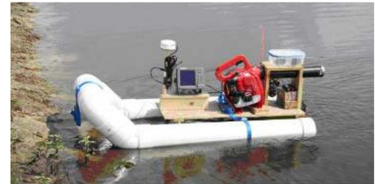
Remote control sludge survey boat using sonar and GPS technology.
